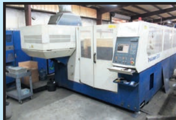
TRUMPF TRUMATIC L3030 4,000W CNC LASER
