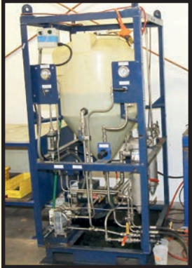
SEVERAL PRESSURE TEST STANDS
