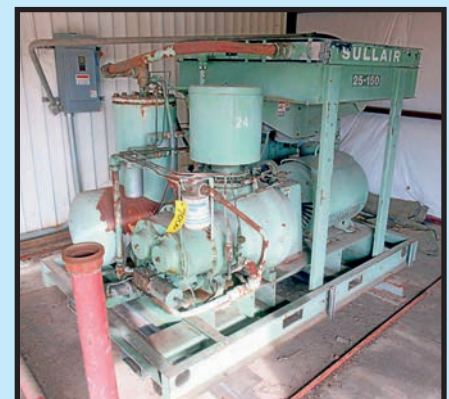
SULLAIR 25 HP ROTARY SCREW AIR COMPRESSOR
