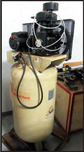
INGERSOLL RAND VERTICAL AIR COMPRESSOR
