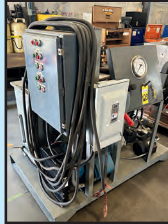
HYDRAULIC POWER PACK
