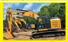
**2012 CAT 320ELRR** SN:TFX00326 powered by Cat diesel engine, equipped with Cab, air, heat, reduced tail swing, 31in. Pads, 34in. Digging bucket w/ thumb, long undercarriage.
