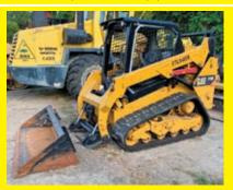
2015 CAT 259D SN:FTL04159 powered by Cat diesel engine, equipped with rollcage, auxiliary hydraulics, 2-speed, auxiliary hydraulics, mechanical quick coupler, 16in. Rubber tracks, 74in. GP bucket.
