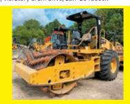
**CAT CP56B** SN:C5P00209 powered by Cat diesel engine, equipped with OROPS, 84in. padsfoot drum, vibratory drum, drum drive, 23.1-26 rubber.
