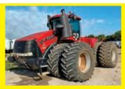
**2014 CASE 580HD STEIGER** SN:ZEF300561 powered by Case IHFPT diesel engine, 580.7hp, equipped with EROPS, air, heat, 16F x 2R full powershift transmission, quad couplers, scraper hitch, front counterweights, 800/70R32 dual tires.
