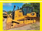
2016 CAT D7E SN:HKA00471 powered by Cat diesel engine, equipped with EROPS, air, heat, Straight blade w/tilt, 3rd valve.
