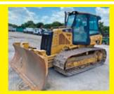
**2008 CAT D5K2LGP** SN:YYY00645 powered by Cat diesel engine, equipped with EROPS, air, heat, 6 way blade, 26in. Pads, Grade Control.
