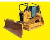
2016 CAT D6NLGP SN:MG500466 powered by Cat diesel engine, equipped with EROPS, air, heat, sweeps & screen, 6 way blade, wide pads, 3-shank rear ripper, Grade Control, new undercarriage from Mustang Cat.
