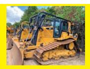
**2015 CAT D6TVPLGP** SN:RAD00901 powered by Cat diesel engine, equipped with EROPS, air, heat, sweeps & screens, 6 way blade, 31in. Pads, Diamond 3-shank rear ripper.
