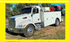
**2012 PETERBILT 337** VN:2NP2HN7X9CM162274 powered by Paccar PX-8 diesel engine, equipped with Eaton 10 speed transmission, power steering, Service body, Stellar 10628 10,000lb crane, hydraulic outriggers, Lincoln 305G Ranger welder, Infinity air compressor, oil tank, dual wheel single axle, 198,190 miles.
