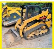
2017 CAT 259D SN:FTL11750 powered by Cat diesel engine, equipped with rollcage, auxiliary hydraulics, 2-speed, auxiliary hydraulics, mechanical quick coupler, 16in. Rubber tracks, 74in. GP bucket, 2,066 hours.
