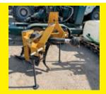
AMCO AD540V DITCHER equipped with 3pt hitch, PTO..
