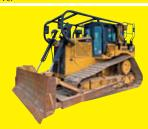
2018 CAT D6TLGP SN:JML00379 powered by Cat diesel engine, equipped with EROPS, air, heat, sweeps, Straight blade w/ tilt, 36in. Pads, Paccar winch.
