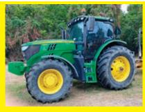
JOHN DEERE 6155R VN:1BW615SRJD028629 powered by John Deere diesel engine, equipped with OROPS, 3pt hitch, PTO, front counterweights, 540/65R28 front rubber, 650/65R38 rear rubber.
