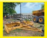
**HOLLY 12FT.** equipped with 12ft. Width, Topcon, 31x13.5-15 tires.
