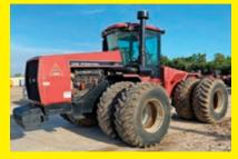
CASE 9280 SN:JEF0032578 powered by Cummins NTA-855-A diesel engine, 375hp, equipped with EROPS, air, heat, quad coupler, 24.5R32 dual tires.
