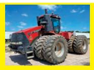
2014 CASE 580HD STEIGER SN:ZEF301517 powered by Case IHFPT diesel engine, 580.7hp, equipped with EROPS, air, heat, 16F x 2R full powershift transmission, quad couplers, scraper hitch, front counterweights, 800/70R32 dual tires.
