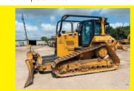
2016 CAT D6NLGP SN:PMG500424 powered by Cat diesel engine, equipped with EROPS, air, heat, sweeps & screens, 6 way blade, 33in. Pads, Diamond 3-shank rear ripper.
