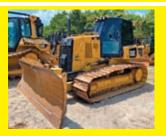
**2017 CAT D6K2LGP** SN:CEL700173 powered by Cat diesel engine, equipped with EROPS, air, heat, 6 way blade, 30in. Pads, Grade Control.
