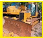
**2017 CAT D5GLGP** SN:RKG00983 powered by Cat diesel engine, equipped with EROPS, air, heat, 6 way blade, Grade Control.
