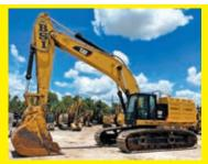
2018 CAT 374FL SN:EBF20017 powered by Cat diesel engine, equipped with Cab, air, heat, reach boom, 13ft 7in stick, 36in. Pads, Cat hydraulic quick coupler, 96in. Digging bucket, long undercarriage, 2,828 idling hours, 5,636 total hours.
