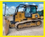
2015 CAT D6K2LGP SN:RST01192 powered by Cat diesel engine, equipped with EROPS, air, heat, sweeps, 6 way blade, 30in. Pads.
