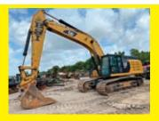
**2016 CAT 349FL** SN:HPD00821 powered by Cat diesel engine, equipped with Cab, air, heat, quick coupler, 72in. Digging bucket, long undercarriage.
