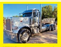
**2011 PETERBILT 388** VN:136747 powered by Cummins ISX-25 diesel engine, 525hp, equipped with Eaton 18 speed transmission, power steering, wet line, 265in. Wheelbase, air lift third axle, triaxle.
