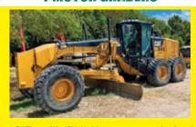
2016 CAT 140M3 SN:N9M00408 powered by Cat diesel engine, equipped with EROPS, air, heat, rearview camera, 14ft. Moldboard, hydraulic sideshift, TIP control, push block, rear ripper, Grade Control.
