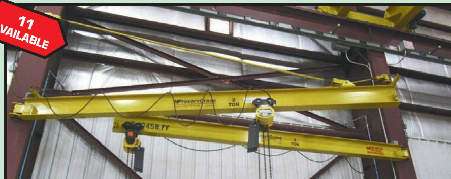
SAMPLE VIEW OF PROSERV 2 T. CAP. X 18' REACH WALL MOUNTED JIB CRANES
