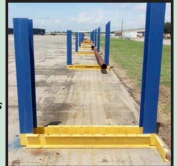
H.D. PIPE RACKS
