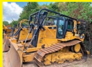
**2015 CAT D6TVPLGP** SN:RAD00901 powered by Cat diesel engine, equipped with EROPS, air, heat, sweeps & screens, 6 way blade, 31in. Pads, Diamond 3-shank rear ripper.
