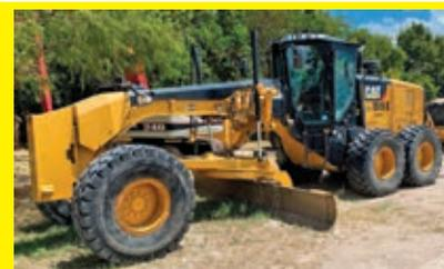
**2016 CAT 140M3** SN:N9M00408 powered by Cat diesel engine, equipped with EROPS, air, heat, rearview camera, 14ft. Moldboard, hydraulic sideshift, TIP control, push block, rear ripper, Grade Control.
