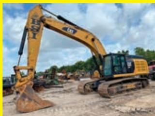
**2016 CAT 349FL** SN:HPD00821 powered by Cat diesel engine, equipped with Cab, air, heat, quick coupler, 72in. Digging bucket, long undercarriage.
