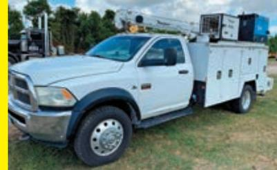
**2012 FORD F550** VN:235441 4x4, powered by Cummins diesel engine, equipped with automatic transmission, power steering, Maintainer service body, Maintainer 6,500lb crane, RC-40 air compressor, Bobcat welder, dual wheel single axle, 255,266 miles.
