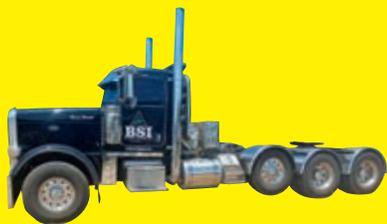
**2011 PETERBILT 388 VN:150014** powered by Cummins ISX diesel engine, 600hp, equipped with Eaton 18 speed transmission, power steering, wet line, 256in. Wheelbase, air lift steerable axle, triaxle.
