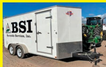
**2020 CARRY-ON 7X16CGRCM** VN:5049 equipped with 7,000 GVWR, 7ft wide, 16ft length, side door, lay down rear door, ST205/75D15C tires, tandem axle.
