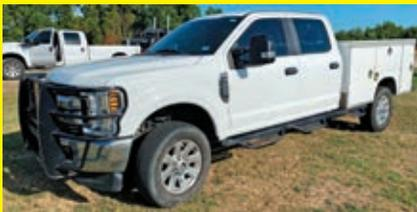
**2018 FORD F350STX** VN:EC70921 4x4, powered by 6.2L gas engine, equipped with automatic transmission, power steering, Royal 8ft. Utility body, 179,804 miles.
