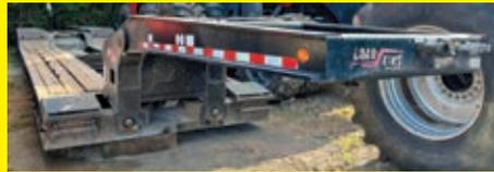
**2012 LOAD KING 554SS** VN:28247 equipped with 55 ton capacity, non-ground bearing, 26ft. well, 9ft. wide, outriggers, rear wheel covers, air ride suspension, aluminum wheels, 275/70R22.5 tires, 2-rear air lift axles, quad axle.
