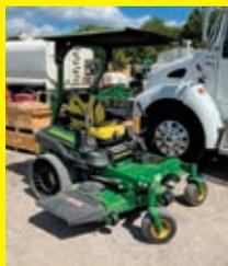
**JOHN DEERE Z930R** SN:70715 powered by gas engine, equipped with 7 Iron Pro 60 deck, zero turn, 45 hours.
