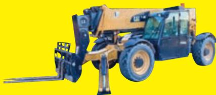
2013 CAT TL1255C SN:DHW00583 4x4, powered by Cat C4.4 ACERT diesel engine, equipped with EROPS, air, heat, 12,000lb lift capacity, 55ft. Reach height, front stabilizers, rotating forks, 400/75-28 rubber.
