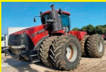
**2014 CASE 580HD STEIGER** SN:ZEF300578 powered by Case IHFPT diesel engine, 580.7hp, equipped with EROPS, air, heat, 16F x 2R full powershift transmission, quad couplers, scraper hitch, front counterweights, 800/70R32 dual tires.
