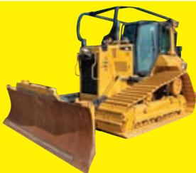
**2016 CAT D6NLGP** SN:MG500466 powered by Cat diesel engine, equipped with EROPS, air, heat, sweeps & screen, 6 way blade, wide pads, 3-shank rear ripper, Grade Control, new undercarriage from Mustang Cat.
