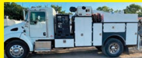
**2007 KENWORTH T300** VN:211995 powered by Paccar PX-8 diesel engine, 330hp, equipped with Eaton 10 speed transmission, power steering, Service body, Autocrane 8,000lb lift crane, Boss BA435 air compressor, Miller Big Blue welder, hydraulic outriggers, 11R22.5 tires, dual wheel single axle.
