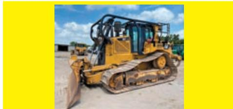
**2015 CAT D6TVPLGP** SN:RAD00773 powered by Cat diesel engine, equipped with EROPS, air, heat, sweeps & screens, 6 way blade, 31in. Pads, Diamond 3-shank rear ripper.
