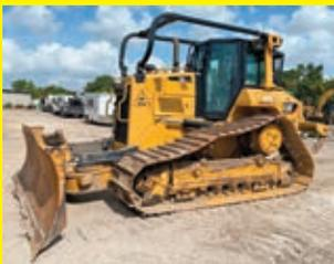
**CAT D6NLGP** SN:CMC500713 powered by Cat diesel engine, equipped with EROPS, air, heat, sweeps & screens, 6 way blade, 33in. Pads, Diamond 3-shank rear ripper, Grade Control.
