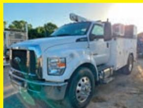
**2015 FORD F650** VN:A00870 powered by 6.7L Power Stroke diesel engine, equipped with automatic transmission, power steering, service body, Autocrane 8,000lb crane, Palfinger PRC 45V air compressor, Miller Bobcat welder, hydraulic outriggers, dual wheel single axle, 93,425 miles.
