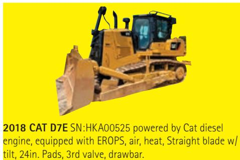
**2018 CAT D7E** SN:HKA00525 powered by Cat diesel engine, equipped with EROPS, air, heat, Straight blade w/ tilt, 24in. Pads, 3rd valve, drawbar.
