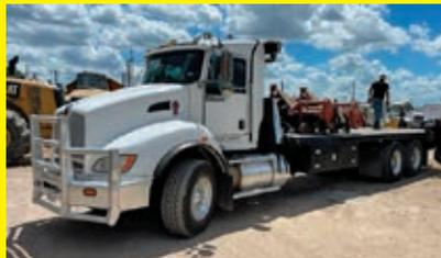
**2012 KENWORTH T440** VN:956363 powered by Paccar PX-8 engine, 330hp, equipped with Allison automatic transmission, a/c, 28ft rolloff body, winch, hydraulic rear hitch, air ride suspension, aluminum wheels, 11R22.5 tires, tandem axle, 187,000 miles.
