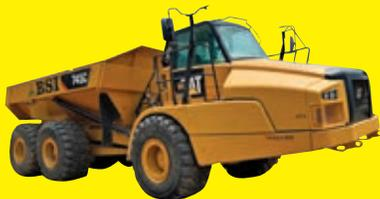
**2017 CAT 745C** SN:TFK01486 6x6, powered by Cat diesel engine, equipped with Cab, air, heat, 45 ton capacity, 875/65R29 rubber.
