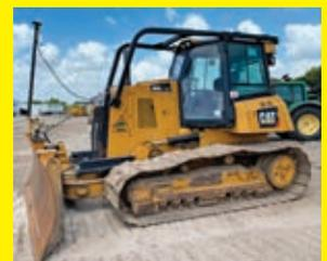
**2015 CAT D6K2LGP** SN:RST01192 powered by Cat diesel engine, equipped with EROPS, air, heat, sweeps, 6 way blade, 30in. Pads.
