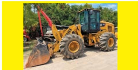
**2013 CAT 938K** SN:SWL01363 powered by Cat diesel engine, equipped with EROPS, air, heat, quick coupler, GP bucket, 28LB-26 skidder rubber.
