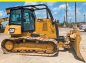
**CAT D6K2LGP** SN:RST0145 powered by Cat diesel engine, equipped with EROPS, air, heat, 6 way blade, 30in. Pads, 3rd valve.
