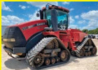
**CASE 550 QUAD TRAC** SN:ZBF128254 powered by diesel engine, 549.9hp, equipped with EROPS, air, heat, 16/FX2R full powershift transmission, 30in. Rubber tracks, quad coupler, front counterweights.
