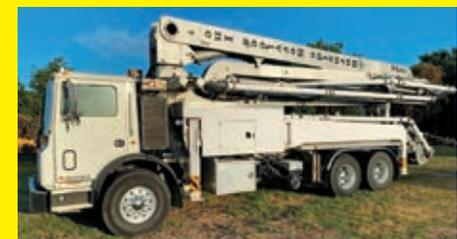
**2012 MACK MRU613** VN:DM009667 powered by Mack MP7 diesel engine, equipped with Eaton 8 speed transmission, power steering, 2012 Alliance JXR37-4.16 pumper (sn:1206), 123ft. 4in. Reach height, tandem axle.
