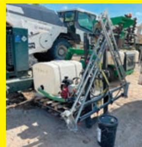
**SPRAYER** equipped with 100 gallon tank, pump, 19ft. spray boom, for ATV utility box.
