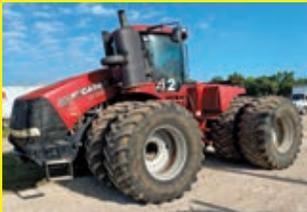
**2015 CASE 580HD STEIGER** SN:ZEF304123 powered by Case IHFPT diesel engine, 580.7hp, equipped with EROPS, air, heat, 16F x 2R full powershift transmission, quad couplers, scraper hitch, front counterweights, 800/70R32 dual tires.
