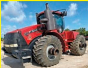
**2015 CASE 580HD STEIGER** SN:ZFF303958 powered by Case IHFPT diesel engine, 580.7hp, equipped with EROPS, air, heat, 16F x 2R full powershift transmission, quad couplers, scraper hitch, front counterweights, 800/70R32 dual tires.
