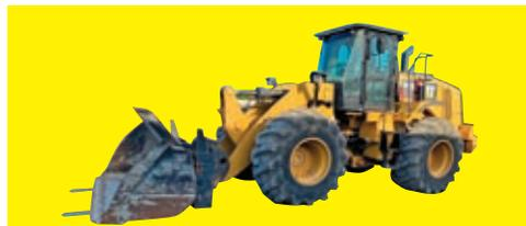
**2015 CAT 950M** SN:EMB00824 powered by Cat diesel engine, equipped with EROPS, air, heat, GP bucket, 345LB-32 skidder rubber. Forks Sell Separately.
