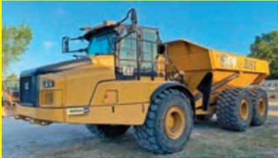
**2018 CAT 745** SN:3T600901 6x6, powered by Cat diesel engine, equipped with Cab, air, heat, 45 ton capacity, 875/65R29 rubber.
