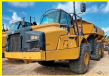
**2015 CAT 740B** SN:T4R03051 6x6, powered by Cat diesel engine, equipped with Cab, air, heat, 40 ton capacity, 29.5R25 rubber.
