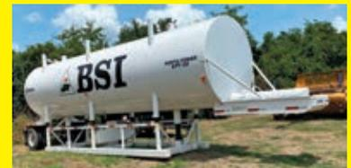
**2019 KLEIN KPT-120** SN:42841 equipped with 12,000 gallon water tank, hydraulic raise, water filler, Honda engine, single axle.
