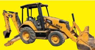
**2017 CAT 420F2** SN:HWC01950 4x4, powered by Cat diesel engine, equipped with OROPS, GP front bucket, 24in. Rear digging bucket.
