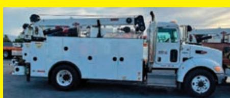
**2017 PETERBILT 337** VN:2NP2HM7X1HM387211 powered by Paccar PX-7 diesel engine, 250hp, equipped with Allison 2500 RDS automatic transmission, power steering, clutch shift PTO, IMT Dominator II 14ft. Service body, IMT 10,000lb crane, 30ft. 10in. horizontal reach, MI-T-M air compressor/generator, welder, lube kit, aluminum rock guards, bumper vise, Line-X bed floor, 21 gallon hydraulic reservoir, manual outriggers, spring suspension, air brakes, 22.5 tires, dual wheel single axle, 70,215 miles.
