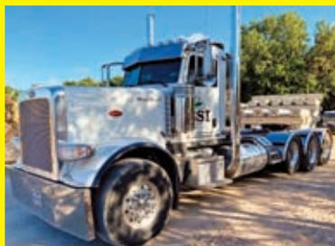
**2011 PETERBILT 388 VN:136747** powered by Cummins ISX-25 diesel engine, 525hp, equipped with Eaton 18 speed transmission, power steering, wet line, 265in. Wheelbase, air lift third axle, triaxle.
