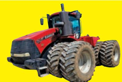
**2016 CASE 580HD STEIGER** SN: ZFF308129 powered by Case IHFPT diesel engine, 580.7hp, equipped with EROPS, air, heat, 16F x 2R full powershift transmission, quad couplers, scraper hitch, front counterweights, 800/70R32 dual tires.
