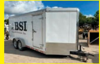
**FOREST RIVER TXCM718TA4** VN:84598 equipped with 12,000lb GVWR, 18ft length, 7ft wide, side door, laydown rear door, 2016 Atlas Copco XAS110 air compressor, powered by Kubota diesel engine, tandem axle.
