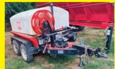
**(2) MULTIQUIP** powered by Honda gas engine, equipped with 500 gallon tank, tandem axle.
