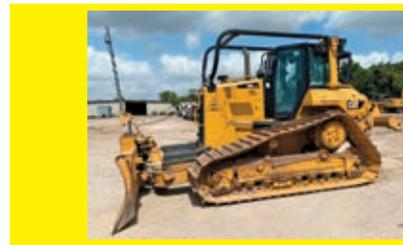
**2016 CAT D6NLGP** SN:PMG500424 powered by Cat diesel engine, equipped with EROPS, air, heat, sweeps & screens, 6 way blade, 33in. Pads, Diamond 3-shank rear ripper.
