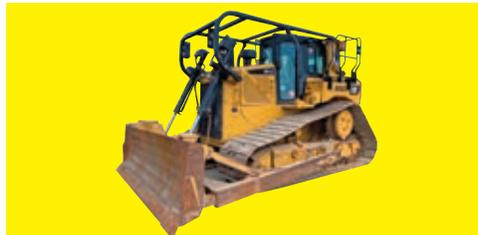
**2018 CAT D6TLGP** SN:JML00379 powered by Cat diesel engine, equipped with EROPS, air, heat, sweeps, Straight blade w/ tilt, 36in. Pads, Paccar winch.
