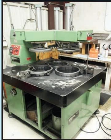
**LAPMASTER 36 W/NORDIC ES-3 ELECTROMAGNETIC CONTROL LAPPING MACHINE**
