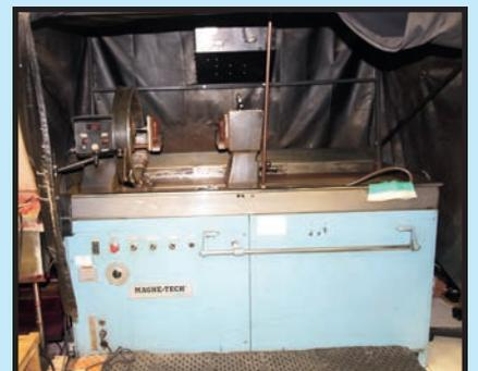
**MAGNE-TECH MDL. 3504 MAGNETIC PARTICLE INSPECTION MACHINE**
