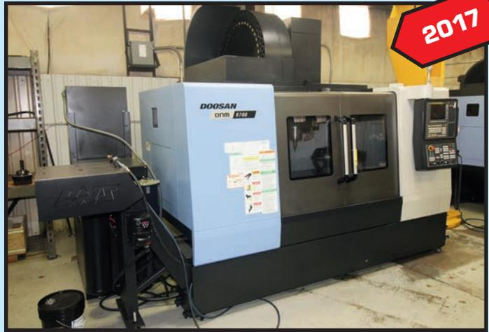
DOOSAN MDL. DNM 6700 4-AXIS VERTICAL MACHINING CENTER
