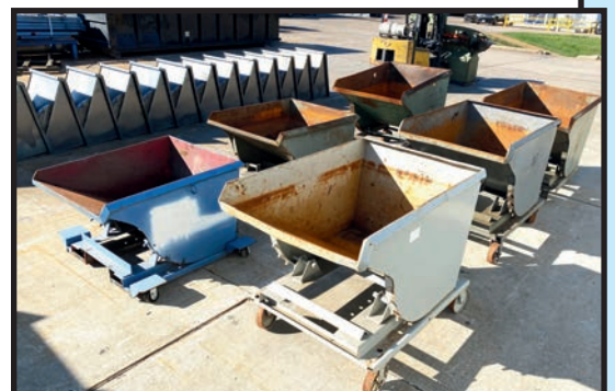
VIEW OF SELF DUMPING HOPPERS
