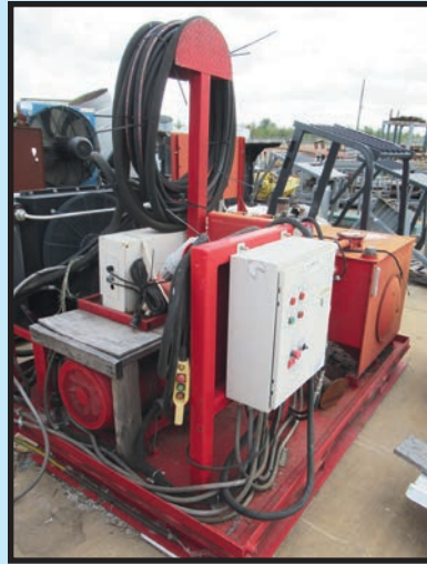
VIEW OF HYDRAULIC POWER UNITS
