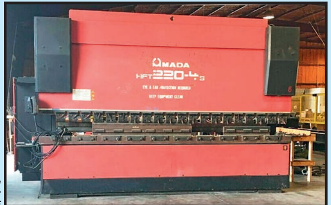
AMADA 200 T. X 168" BED HFT-220-4S CNC PRESS BRAKE
