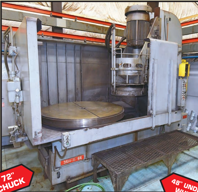
BLANCHARD MDL. 36HD-66 VERTICAL ROTARY SURFACE GRINDER
