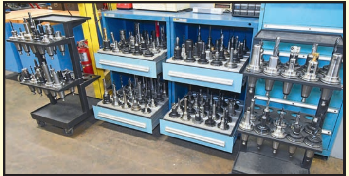
PARTIAL VIEW OF CAT-40 AND CAT-50 TOOL HOLDERS
