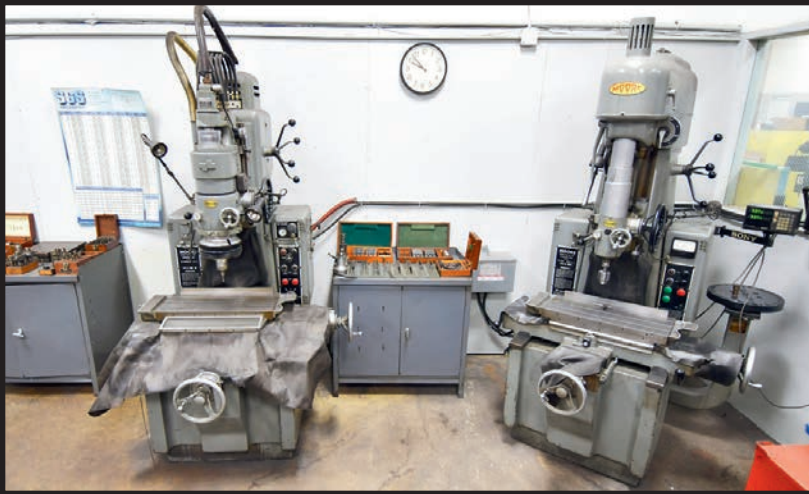
VIEW OF MOORE JIG GRINDER AND BORER
