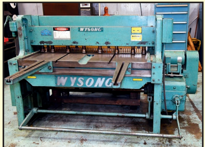
WYSONG 12 GA. X 52" CAP. MECHANICAL SHEAR
