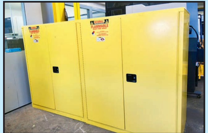
FLAMMABLE MATERIAL STORAGE CABINETS
