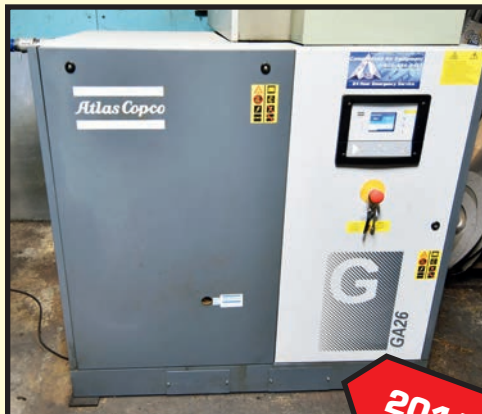
ATLAS COPCO 35 HP ROTARY SCREW AIR COMPRESSOR
