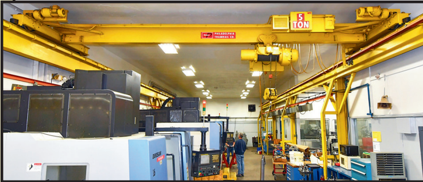
PHILADELPHIA TRAMRAIL 5 T. CAP. OVERHEAD BRIDGE CRANE SYSTEM
