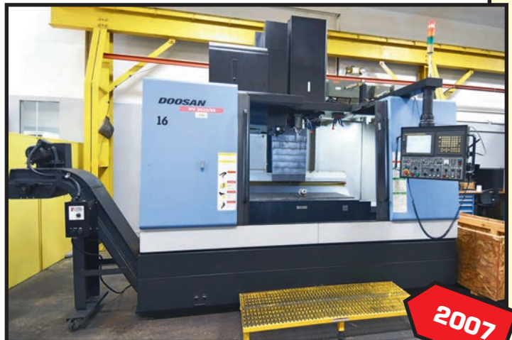
DOOSAN MDL. MV5025/50 4-AXIS VERTICAL MACHINING CENTER
