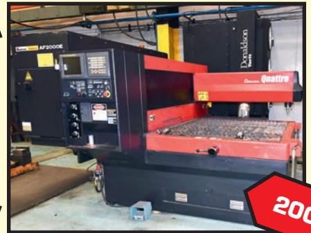
AMADA QUATRO CNC 4' X 4' SHEET CAP. LASER
