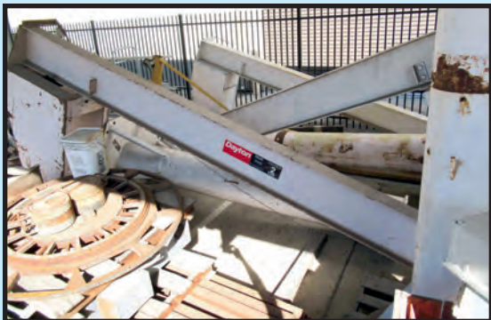
(3) DAYTON 10'H. X 12' REACH X 2-TON PEDESTAL JIB CRANES
