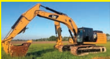
2016 CAT 336FL SN:RKB10687 powered by Cat diesel engine, equipped with Cab, air, heat, hydraulic quick coupler, digging bucket, long undercarriage.
