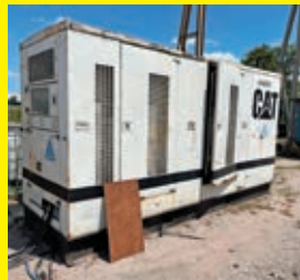
LOT 139: CAT SR4B GENERATOR SN:E46PW813 powered by Cat 3304 diesel engine, equipped with 175KW, skid mounted.
