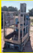
2015 GENIE GR-20 SN:GR15-37119 electric powered, equipped with 20ft. Platform height, slide out deck, 500lb lift capacity, 395 hours.
