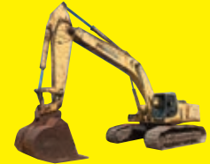
LOT 108: KOMATSU PC600LC-6 HYDRAULIC EXCAVATOR SN:11058 powered by Komatsu diesel engine, equipped with cab, air, heat, 10ft. stick, 36in. pads, hydraulic coupler, Hensley 6 yard digging bucket, long undercarriage.
