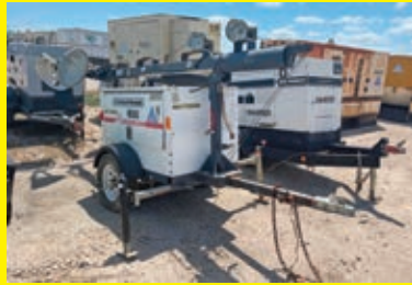
LOT 119: MAGNUM PRO MLT3060M LIGHT PLANT SN:1401795 powered by diesel engine, equipped with 4-1,000 watt lightbulbs, 6KW, trailer mounted.
