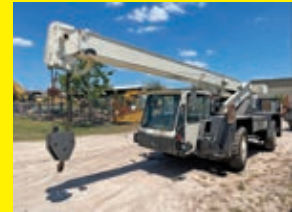
LOT 130: KOEHRING LRT110 ROUGH TERRAIN CRANE SN:98798 powered by Cummins diesel engine, equipped with Cab, 7.5 ton capacity, 36ft. reach.
