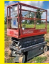
2014 SKYJACK SJIII3219 SN:22067462 electric powered, equipped with 19ft. Platform height, slide out deck, 500lb lift capacity, 163 hours.
