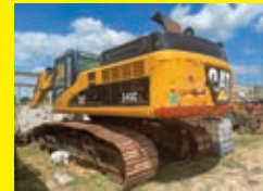
LOT 111: CAT 345CL HYDRAULIC EXCAVATOR SN:TDG00362 powered by Cat diesel engine, equipped with Cab, air, 36in. pads, digging bucket, long undercarriage. No hydraulic pump, not running.
