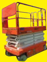
2017 SNORKEL S4732E SN:S4732E-04-170200989 electric powered, equipped with 32ft. Platform height, slide out deck, 500lb lift capacity, 125 hours.
