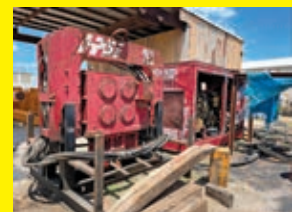
LOT 133: HPSI 260 PILE DRIVER SN:HPS0959 powered by Cat 3406 hydraulic power pack, 355hp, 5,000PSI, equipped with 2,600 in lb exciter, all skid mounted.
