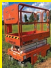
2017 SNORKEL S3215E SN:S3215E-04-000002 electric powered, equipped with 15ft. Platform height, slide out deck, 500lb lift capacity, 155 hours.
