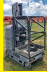
2013 JLG 20MVL SN:0130019844 electric powered, equipped with 20ft. Platform height, slide out deck, 500lb lift capacity.
