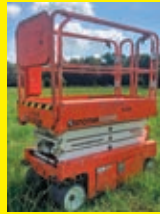
(2) 2019 SNORKEL S3219E electric powered, equipped with 19ft. Platform height, slide out deck, 500lb lift capacity.
