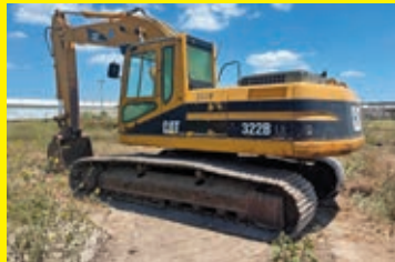
LOT 123: CAT 322BL HYDRAULIC EXCAVATOR SN:1YS01415 powered by Cat diesel engine, equipped with Cab, air, heat, reach boom, 10ft. stick, 32in. pads, digging bucket, long undercarriage.
