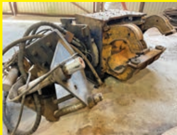
LOT 142: 2004 SHEET PILE DRIVER SN:04U166 powered by John Deere 4045 hydraulic power pac, equipped with excavator mount, hydraulic driven.
