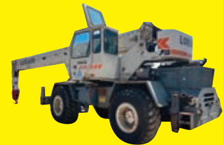
LOT 131: KOEHRING LRT275D ROUGH TERRAIN CRANE SN:79962 powered by diesel engine, equipped with Cab, 27.5 ton capacity, 72ft. reach.
