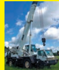
P & H S35 SN:35224 powered by Deutz BF6L-913 diesel engine, equipped with powershift transmission, 80ft. Reach height, (4) sheave hook & block, (4) outriggers, 16 x 24 rubber.
