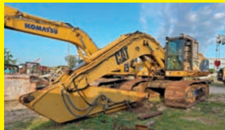
LOT 144: CAT 350L HYDRAULIC EXCAVATOR SN:9FL00929 powered by Cat diesel engine, equipped with Cab, reach boom, stick, 36in. pads, long undercarriage. Unit not running.
