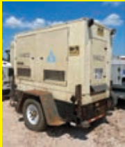
LOT 115: KOHLER 20RE0ZJB GENERATOR SN:788374 powered by diesel engine, equipped with 23KW, trailer mounted.
