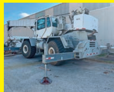
LOT 153: TEREX RT555 ROUGH TERRAIN CRANE SN:16402 powered by diesel engine, equipped with Cab, 55 ton capacity, 110ft. reach, dual winch, 26.5-25 rubber.
