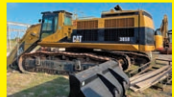
LOT 112: CAT 385BL HYDRAULIC EXCAVATOR SN:ANS00333 powered by Cat diesel engine, equipped with Cab, air, heat, 34in. pads, hydraulic coupler, digging bucket, long undercarriage.
