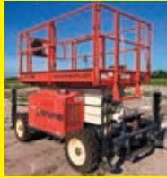
2015 SNORKEL S2770RT SN:S2770RT-07-000144 4x4, electric powered, equipped with 27ft. Platform height slide out deck, rough terrain tires.
