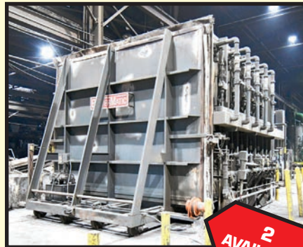
BEAVERMATIC 12'W. X 12'L. X 8'H. GAS FIRED CAR BOTTOM FURNACE
