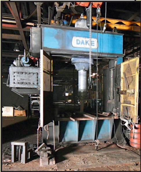
STRAIGHTNING PRESS DAKE 300 T. CAP. HYDRAULIC STRAIGHTENING PRESS.
