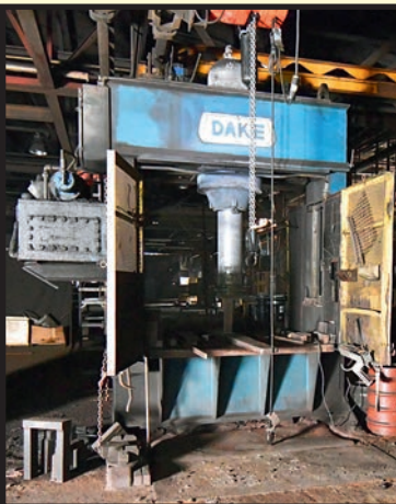
DAKE 300 T. HYDRAULIC STRAIGHTENING PRESS
