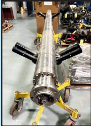
SUBMERSIBLE DOWNHOLE PUMP ON ROLLER STANDS
